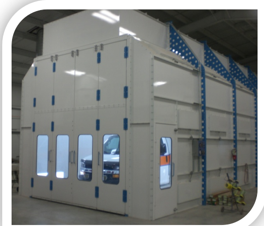
Figure 2: Enclosed paint booth
