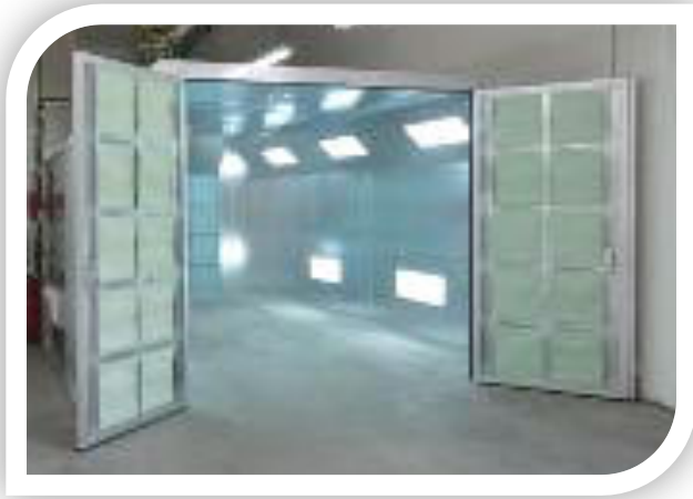
Figure 3: Open faced paint booth with filtered doors
