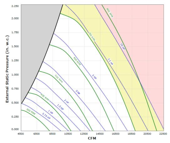
$\label{eq:max_size_able_RPM} \textbf{Max Sizeable RPM = 850 RPM. Curve shown extended beyond this point for reference only.}$
